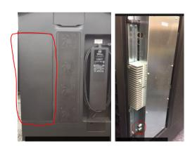
Now, to remove this panel, you have to open sliding door and remove four screws. Please see below picture.
