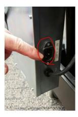
If direct connection of power cord does not power up the cart, this means that controller box might need to be replaced.
