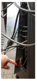
But right now, the controller box is attached to the frame of the cart. You need to remove two more screws on left hand side edge first.
